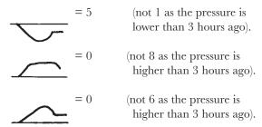
5. When the trace is not steady but the 3-hour pressure change is zero, use code figure 0 or 5 as appropriate for the last part of the trace (code figure 4 is only used when the trace is absolutely steady).
