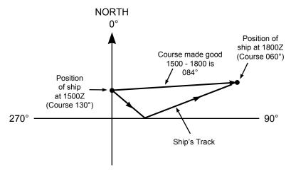
In this example, the ship has altered course during the past three hours, so course made good (084°) differs from the actual course at the time of observation (060°).  $084^{\circ}$  is approximately eastward, so  $D_s$  is coded as 2.
