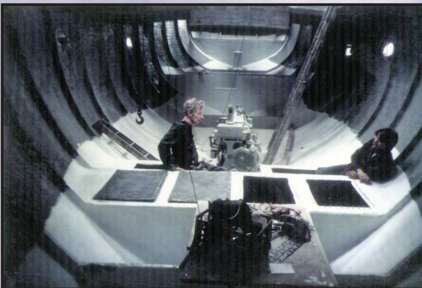
Bob Mason and his son-in-law putting the engine and water tanks inside the empty hull.
