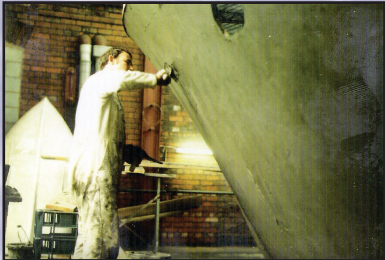
Applying the cement to the outside of the armature.
